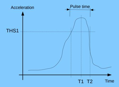
The pulse is a short time peak of the acceleration on one axis
